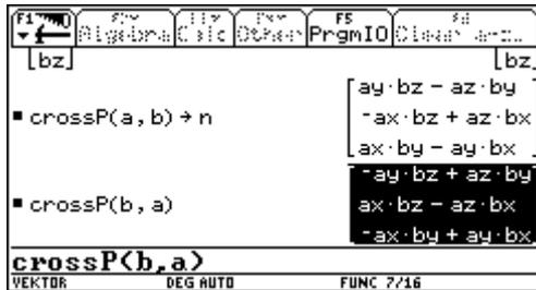
Calculator screen showing the cross product of vectors  $a$  and  $b$ . The result for  $\text{crossP}(a, b)$  is  $\begin{bmatrix} ay \cdot bz - az \cdot by \\ -ax \cdot bz + az \cdot bx \\ ax \cdot by - ay \cdot bx \end{bmatrix}$ . The result for  $\text{crossP}(b, a)$  is  $\begin{bmatrix} -ay \cdot bz + az \cdot by \\ ax \cdot bz - az \cdot bx \\ -ax \cdot by + ay \cdot bx \end{bmatrix}$ . The function name is  $\text{crossP}(b, a)$ .
