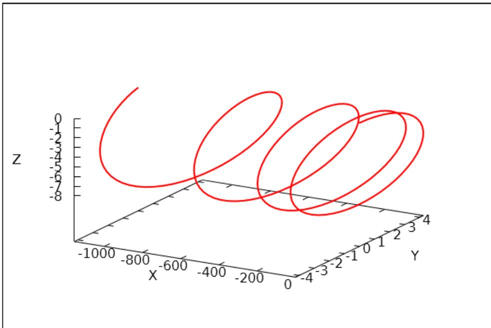
V.7 Solve the equations of motion for a charged particle of mass  $m$  and charge  $q$  moving in an oscillating electric field  $\vec{E} = (E \cos(\omega t), -E \sin(\omega t), 0)$ , where  $\omega = \frac{qB}{m}$ , and a uniform and constant magnetic field oriented perpendicular to this electric field  $\vec{B} = (0, 0, B)$ . Take as initial conditions  $\vec{r}_0 = (0, 0, 0), \vec{v}_0 = (0, 0, 0)$ .
