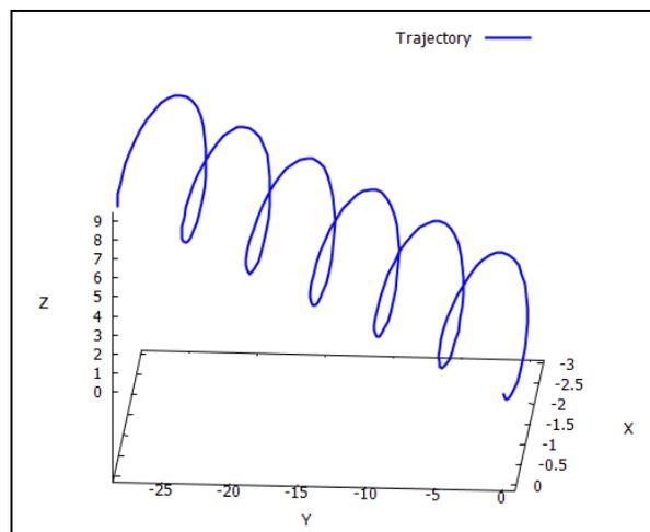
**V.6** Calculate the trajectory of a particle of mass  $m$  and electrical charge  $q$  moving in a constant electric and magnetic field which are oriented in opposite direction to each other. Take this problem as an exercise.
