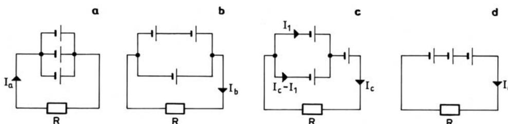
The other possible ways of connecting the cells involve different polarization of the cells, and are thus less favourable.
