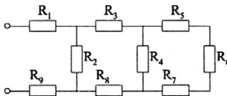
Give the numerical result for the total resistance for  $R_1 = 2\Omega$ ,  $R_2 = 3\Omega$ ,  $R_3 = 2\Omega$ ,  $R_4 = 3\Omega$ ,  $R_5 = 2\Omega$ ,  $R_6 = 3\Omega$ ,  $R_7 = 2\Omega$ ,  $R_8 = 2\Omega$  and  $R_9 = 2\Omega$ .
